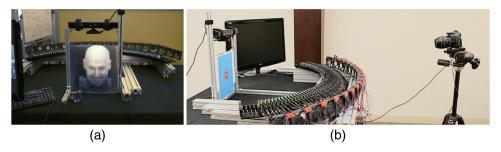
**Fig. 3** (a) Photograph of our rear-mounted projector array setup. (b) Photograph of the calibration setup for front-mounted projector array. To compute relative projector alignment, we sequentially correspond a virtual AR marker generated by each projector with a printed AR marker.
