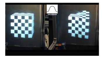
**Video 5** Assuming a constant viewer height per projector frame causes image tearing and distortion (right). Per-vertex height interpolation allows for a consistent perspective (left) [URI: http://dx.doi.org/10.1117/1.JEI.23.1.011005.5].
