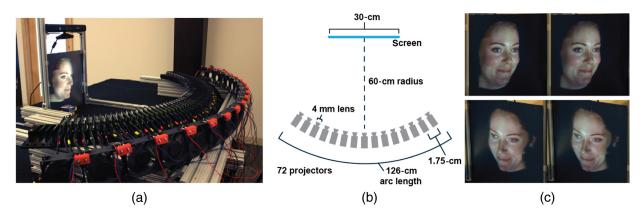
**Fig. 1** (a) A three-dimensional (3-D) face is shown on our autosteroscopic 3-D projector array. The display combines both autostereoscopic horizontal parallax with vertical tracking to generate different horizontal and vertical views simultaneously over a full 110-deg field of view. (b) Diagram showing the dimensions of the display. (c) 3-D stereophotographs of a human face. The stereopairs are left–right reversed for cross-fused stereoviewing.
